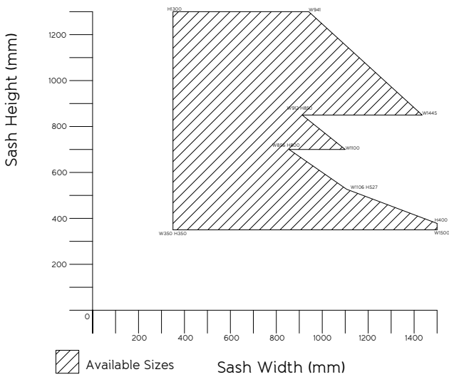
Top Hung Available Sash Dimensions 30kg Glazing Weight (Generic Triple Glazing)
