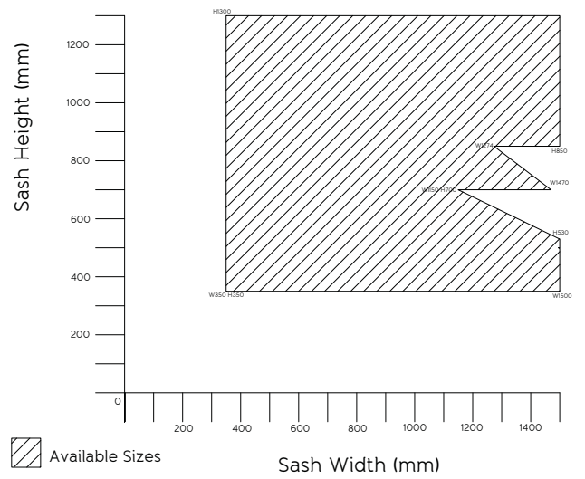
Top Hung Available Sash Dimensions 20kg Glazing Weight (Generic Double Glazing)
